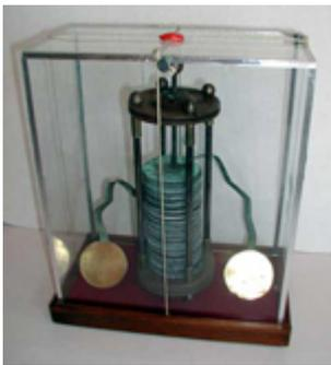
In the year 1800, Alessandro Volta made a battery using multiple layers of silver, paper, and cloth soaked in salt and zinc. The electrochemical series concept which ranks the potential produced when different metals come in contact with an electrolyte. This is where the term volts comes from.
